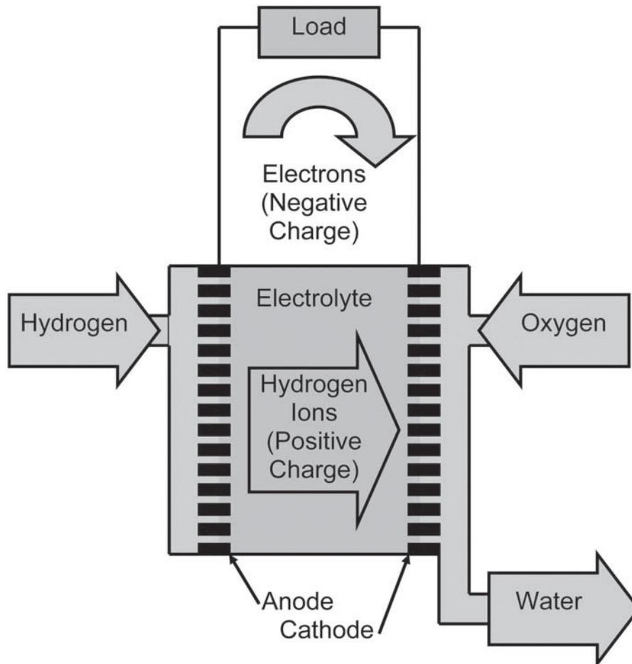
Figure 12-4 - Schematic of basic hydrogen-oxygen fuel cell operation.
