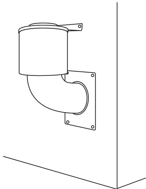
*Figure 7-9 - A specially designed dryer vent hood will reduce air leakage into the house when the dryer is not running. Conventional hoods often allow significant leakage, increasing your heating or cooling bills.*
