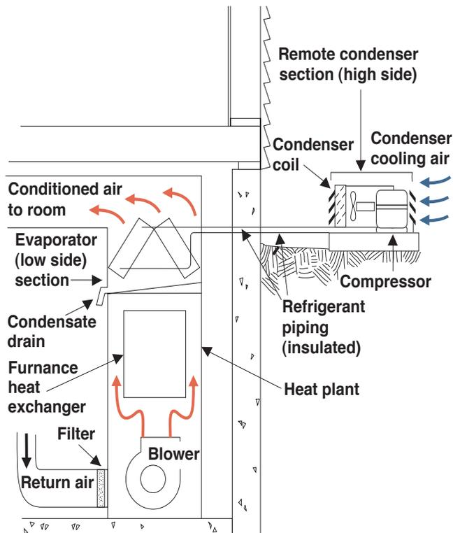
Figure 5-4 - Schematic of air-to-air heat pump
