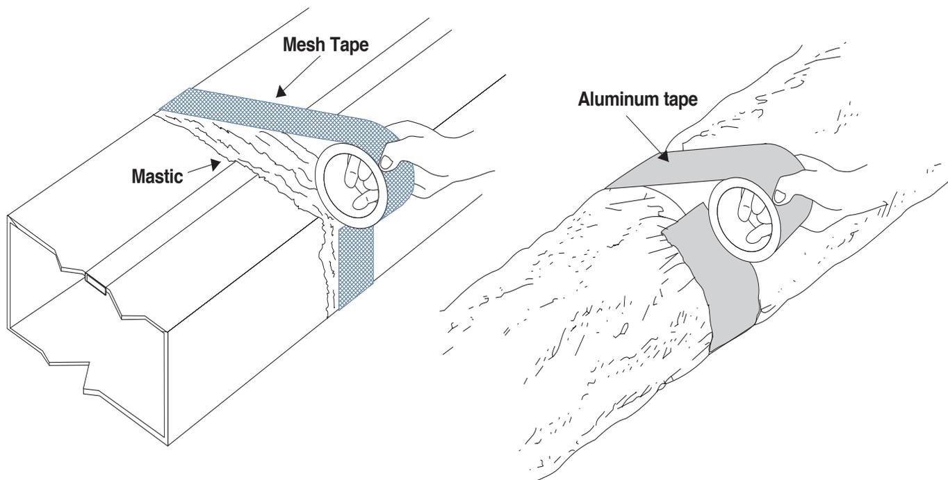
Figure 5-8 - Sealing ducts against air leakage
