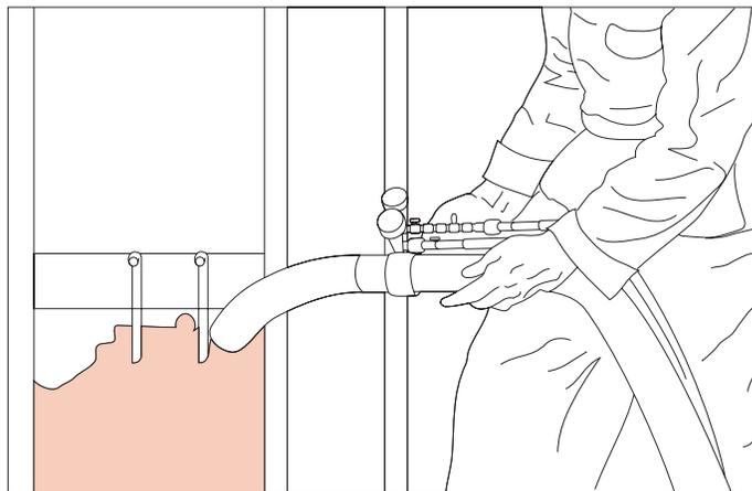
*Figure 3-5 - One unique method for installing either loose-fill fiberglass or cellulose in walls is called the "blow-in-blanket" or "BIB" system.*
