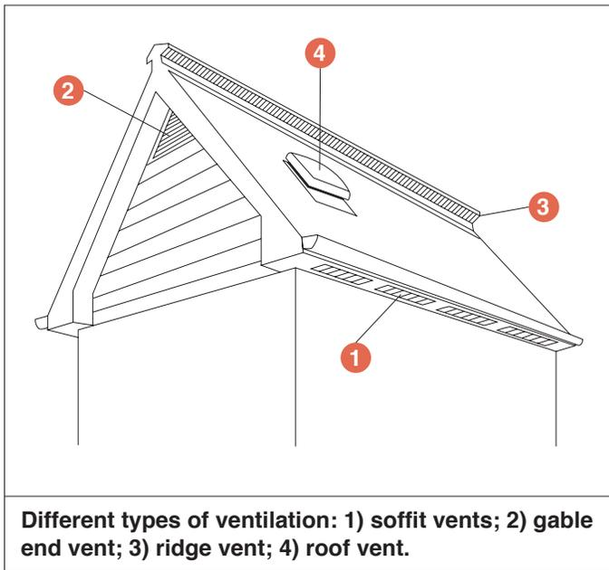
Figure 3-10 - Attic ventilators
