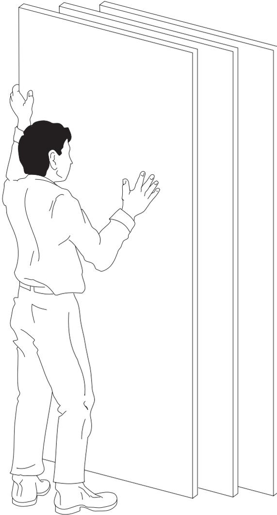
*Figure 3-3 - Rigid foam insulation is made from several different types of plastic foam, each with a different R-value. The most common application for rigid foam is as exterior insulative wall sheathing. Some rigid foam insulation has the significant advantage of being resistant to water, and so is the best insulation for below grade foundation insulation.*
