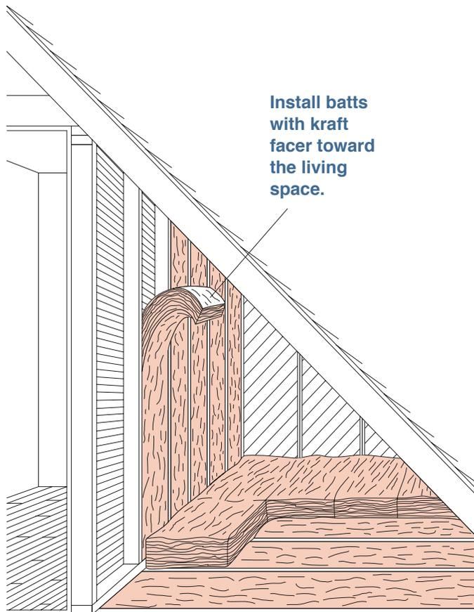
Figure 3-15 - In Cape Cod style homes, where a knee wall separates the second story from an unheated attic space, install batts in the stud cavities.
