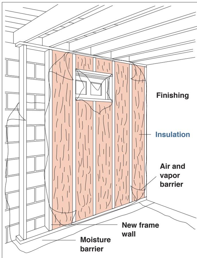
Figure 3-16 - Framed wall insulated with batts.
