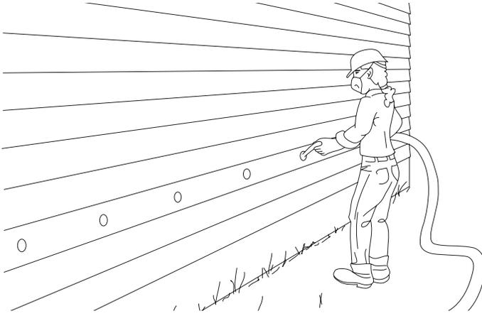
Figure 3-22 Blow-in fiberglass sidewall insulation
