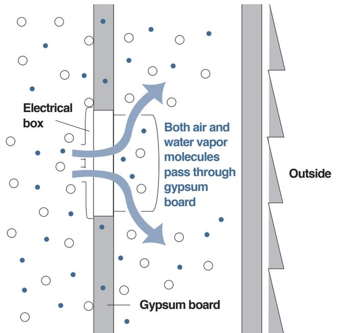
to install a "vapor retarder" (sometimes called a "vapor barrier") on the warm side of the insulation to prevent vapor diffusion into the wall cavity or attic. A vapor
