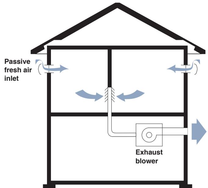
Figure 10-5 - A typical “exhaust-only” ventilation system.
