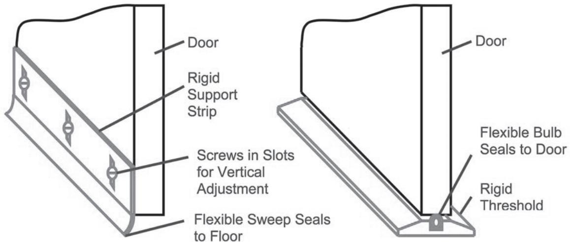
Figure 4-17 – Door Sweep and Vinyl Bulb Threshold
